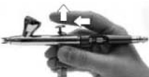
Move the trigger forward to stop paint
